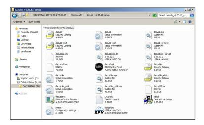
Place the installation disk you received with your CD9 into your computer and double click the SETUP icon. The disk should auto load and start the install function; follow the on screen prompts as you install the DAC USB Audio device drivers.
