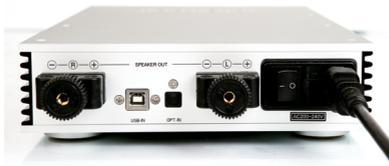
Figure 6. AC Power Cable Connection
