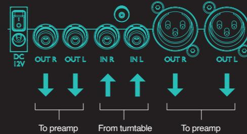
Once Huei is connected, do not switch your preamp/amplifier 'on' until the volume is at its lowest setting. Next, turn Huei 'on' and select the appropriate settings for your cartridge as explained below. With the settings correct, select the lowest gain setting on Huei (white), before turning connected equipment 'on'. Next, select the appropriate input on your preamplifier, begin playing the source and gradually increase the gain/volume to a comfortable level.
