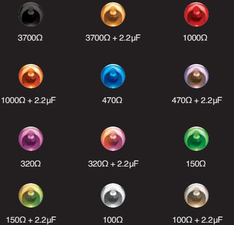
**NOTE: IMPEDANCE CANNOT BE CHANGED WHEN IN MOVING MAGNET MODE. PRESS AND HOLD THE MM/MC BUTTON TO ACTIVATE MOVING COIL MODE. WARNING! PLEASE MUTE OR LOWER THE VOLUME OF YOUR PREAMPLIFIER BEFORE CHANGING IMPEDANCE.**
