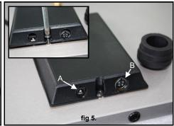
To connect your turntable use **only the supplied wall plug power supply** directly into the jack socket on the back of the new cover tray. (fig 5. A) The Secondary input (fig 5. B) is for connection of the Rega TT PSU which offers electronic speed change and even greater noise reduction and stability. (sold separately). **WARNING:** Socket A and Socket B should never be connected simultaneously, when using the TT-PSU the power supply plug supplied with this kit is no longer required.
