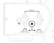
the right line phono sockets. **Note:** The unit connected to the right line phono sockets can be any 'line level' source. However, if connecting an external phono stage (such as the Rega Fono or Aria) it is recommended to use this input as it incorporates isolated grounding to reduce noise and will improve performance.
