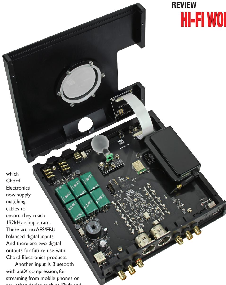
**The illuminated volume ball on a shaft at front, connected to green potentiometer behind. Six green super-capacitors (left) bolster the power supply. At right is the Bluetooth radio module. At centre the square black FPGA chip that holds the WTA filter and DAC.**
